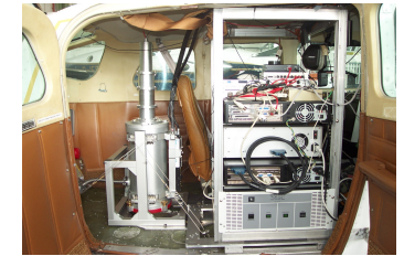
Portable Lidar System (POLIS) Meteorologisches Institut University München
